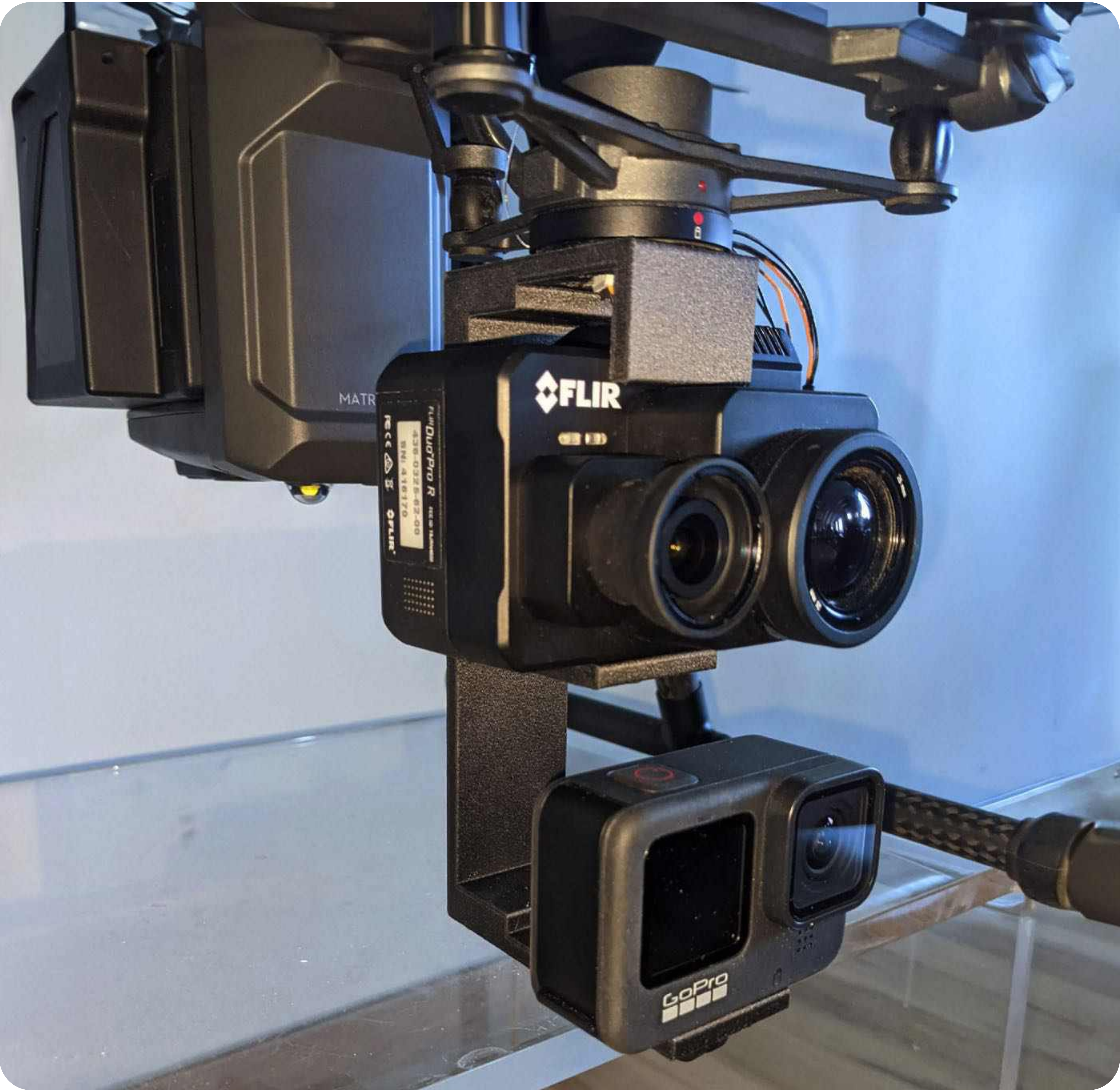
Part of the Dragontech platform incorporates the LIDAR, Multi-Spectral Spectral Sensors, and a controller attached to an enterprise drone via mounts 3D printed on the MakerBot METHOD X using Nylon Carbon Fiber.
