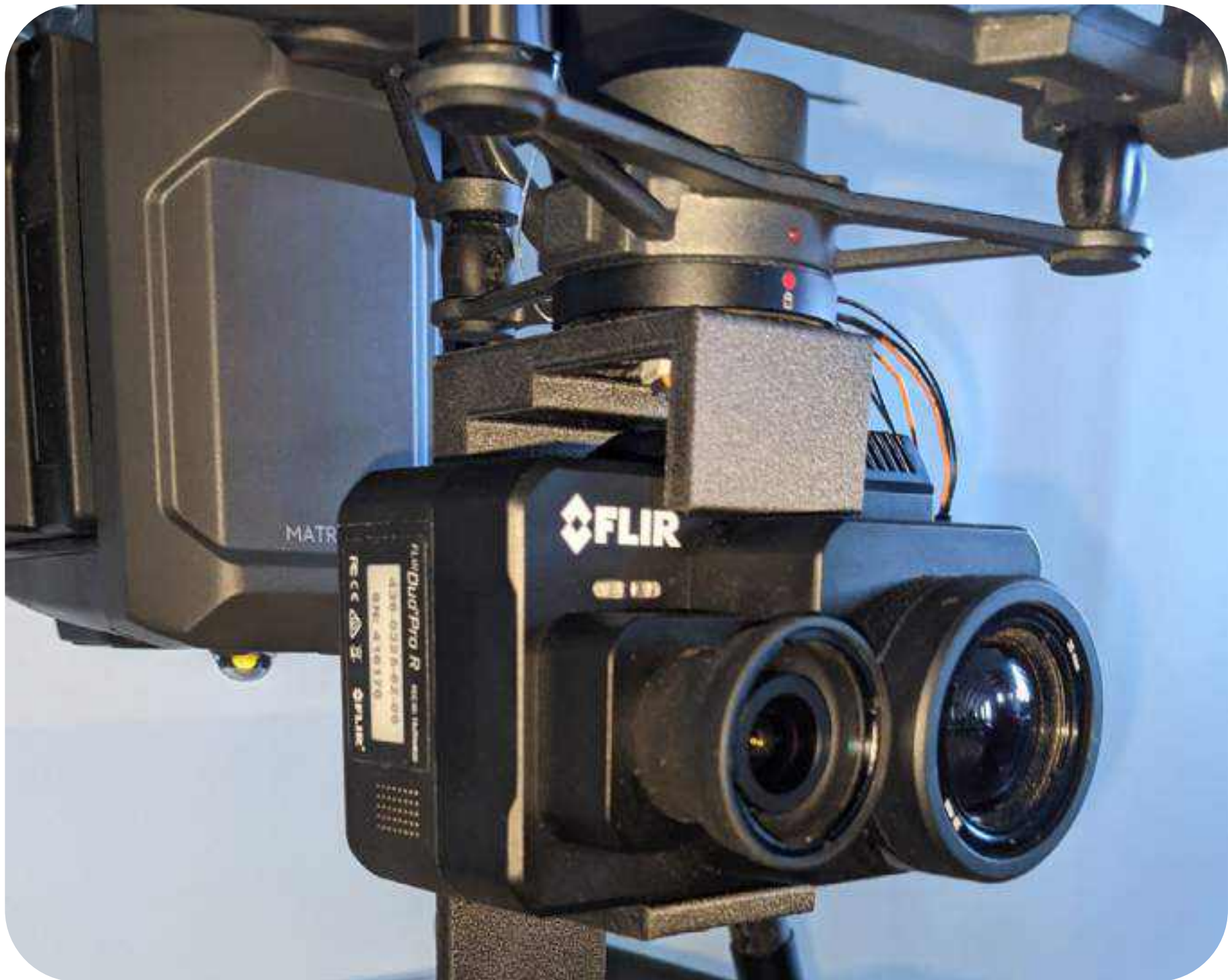
Part of the Dragontech platform incorporates the LIDAR, Multi-Spectral Spectral Sensors, and a controller attached to an enterprise drone via mounts 3D printed on the MakerBot METHOD X using Nylon Carbon Fiber.
