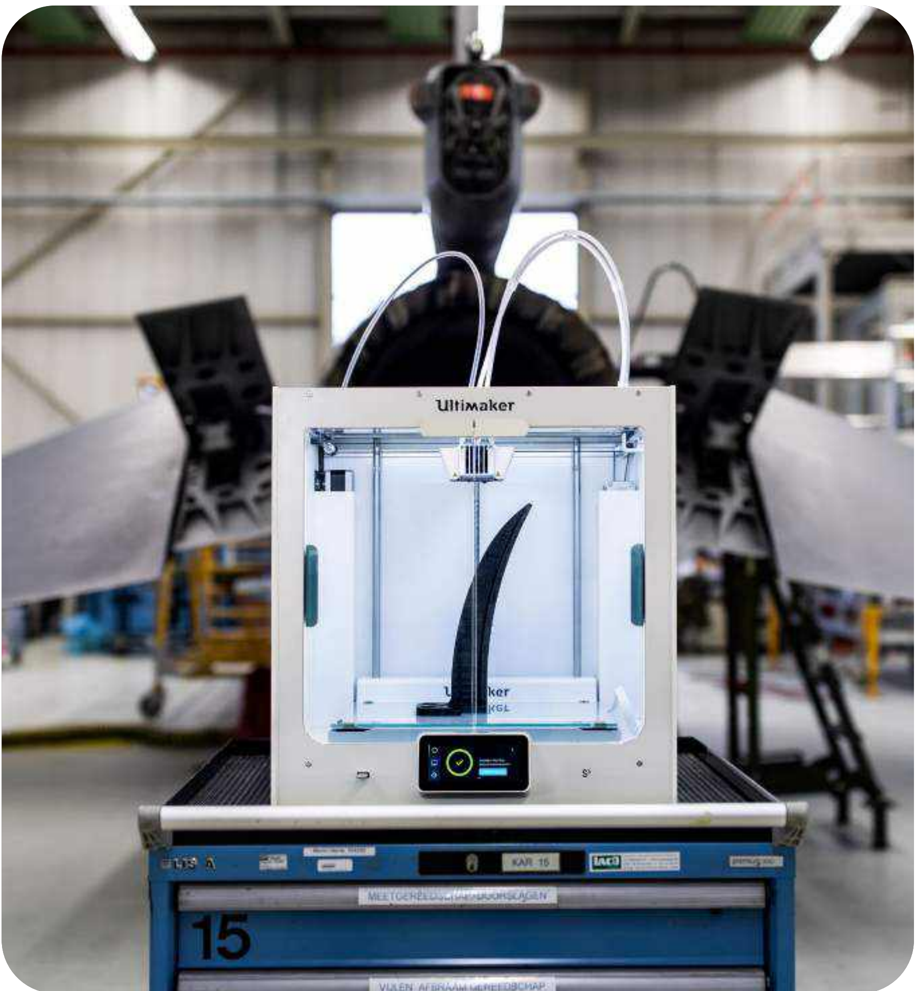
The Royal Netherlands Air Force utilizes UltiMaker 3D printers to produce custom tools for the maintenance of their Chinook, Apache, NH90, and F16 aircraft.
