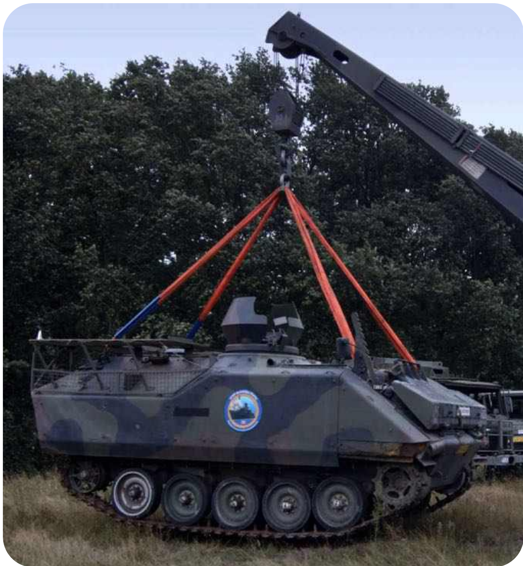
The Royal Dutch Navy proves the material performance of a 3D printed winch link by lifting a 12-ton M113 armored personnel carrier. The link was printed in carbon fiber composite using the UltiMaker S5 3D printer.
